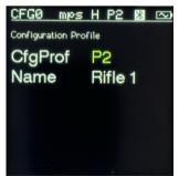
• There are 8 (P0..P7) configuration profiles. Each profile contains a separate and a complete set of device settings.
